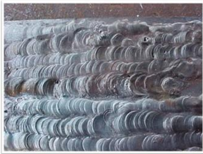
Figure 7.23 unacceptable weld profiles
